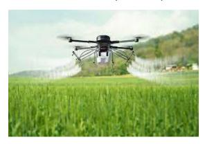
Sprayers are essential in agriculture, since they apply products that control weeds, pests, and diseases. In recent years, drone sprayers have gained popularity due to advantages asso ciated with their flexibility in application timing, ability to operate without being constrained by ground conditions, and ease of deployment.
